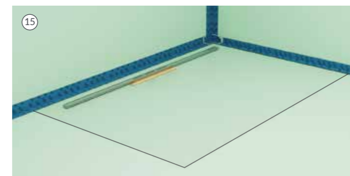
15. Install the full waterproofing course of the shower cabin according to the selected system, e.g. the recommended WIPER Tanking Kit. Directly after applying the liquid waterproofing membrane around the drain base, place the drain channel in its final position on the base.
