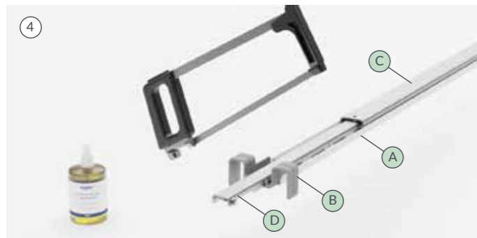
4. Trim the drain grate symmetrically from both its ends by the same length as the drain channel was trimmed; this should result in the grate length 28 mm shorter than the trimmed channel. A – Installation guide piece (for temporary use) B – Cutter for the shower drain channel, grate, and guides C – Shower drain channel D – Grate
