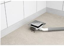
Connect the gulley to the drainage system and set the height using the adjustable legs (optional additional payment) so that the upper edge of the frame is approximately 1mm below the finished surface level of the shower.
