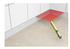
Set the level of the finished shower floor surface and mark it on the wall in the area where the gulley will be fitted (allow for the slope of the shower sur-face).
